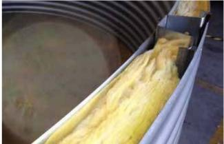
Double sheet plus insulation material: Insulation material is added between sheets. The most common materials are polyurethane foam and fibreglass wool.
