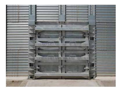
**Bobcat door** opening is ideal for high-capacity silos which are unloaded using light Bobcat machinery so the product residual slope is emptied. It is made with a rigid frame featuring pillars that transmit the loads to the ground and horizontal reinforcements.
