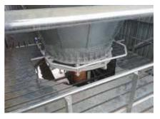
The **vibrating bottom** helps to unload the products stored in hopper silos with poor flow characteristic like flour, granulated poppy, small shells, carbonate, soya beam meal, etc. Recommended for silos with a 60° cone that is reinforced to support the vibration. System is available in different diameters and we
