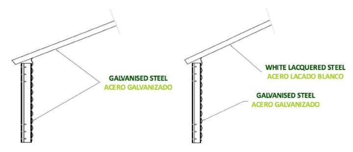
2. Double sheet in wall ring. It can be installed in wall rings or cones (in the case of hopper silos).
