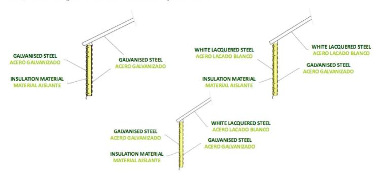
**4. Single sheet + Double roof.** Combination of the first system and double sheet in roof.
