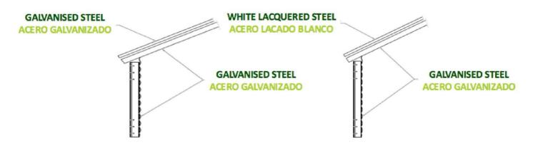
**5. Single sheet + Double roof + Insulation material.** Combination of the first system and double sheet in roof with interior insulation material.
