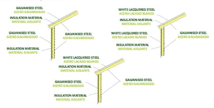
**9. Double sheet in cone.** Enclosure attached to the legs of hopper silos to reduce heat absorption.
