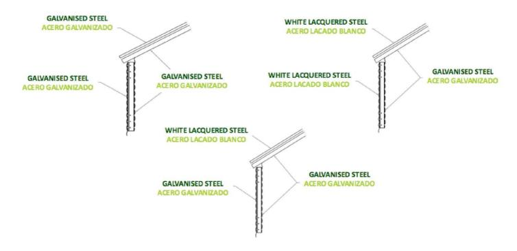
**7. Double sheet + Double roof with insulating material.** Sixth system including interior insulation material only on roof.
