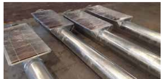
Tubular conveyor with hopper
