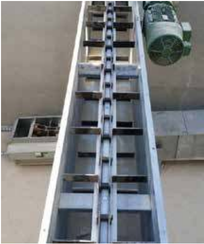
Industrial chain conveyor
